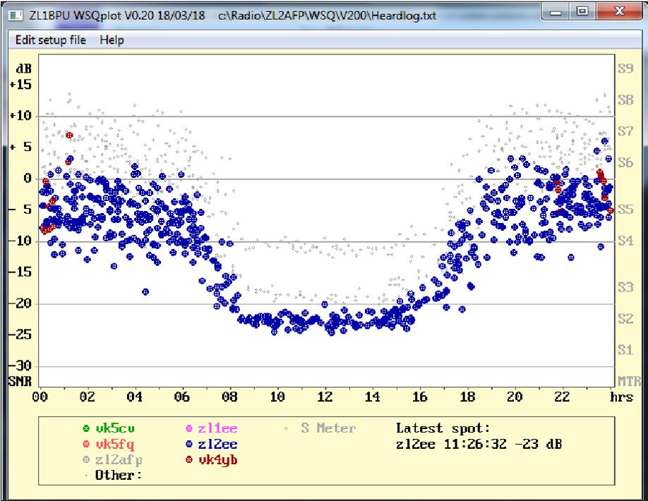
Fig. 79. WSQPlot showing optional S-meter readings
