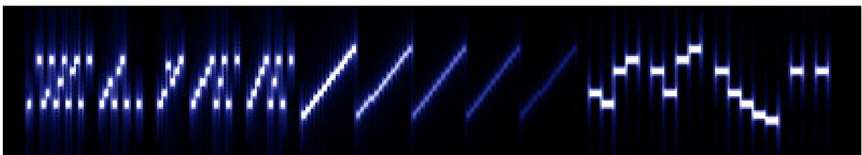
Fig. 50. Multi-mode transmission – 'ZL1EE' in CASTLE on the right.
