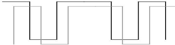
Fig. 15. The effect of multi-path timing and Doppler on an RTTY Signal
